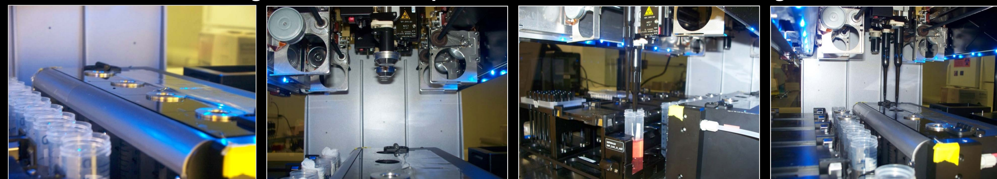
Fig. 4: STARlet manipulations for culture media exchange
